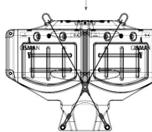
316 grade stainless steel moulded-in tie bars with 2 large integrated lifting and mooring eyes
